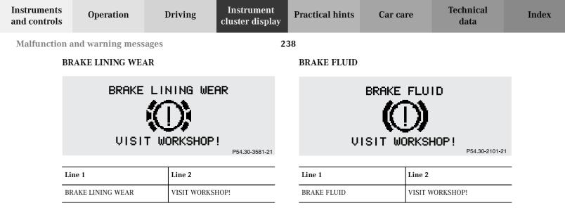
When this message appears during braking, it indicates that the brake pads are worn down.
